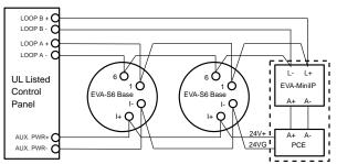
If the AUX. supply circuit needs to be monitored to detect short circuit or open circuit, connect PCE (End-of-line supervision module) to the end of the AUX. supply circuit and EVA-MinilP to SLC.
