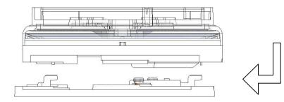
To release, push Release Tool into holes in rim of sounder unit and slide the product in the reverse direction.
