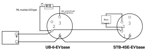
Auxiliary terminal RIL current limited to 3mA. Base control is not current limited as the auxiliary equipment provides the limiting. If the +ve supply for the auxiliary equipment is taken from the EV loop, care must be taken to not cause corruption of the EV protocol by excessive current draw.
