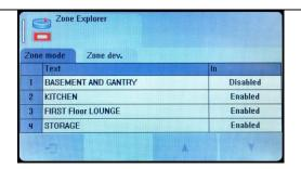
When zones have been disabled, the LCD display changes from SYSTEM NORMAL to Disablement/Test. The screen shows:-
