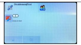
As devices are tested, the screen changes to show the recent tests. Use the arrow to scroll to view older tests if required.
