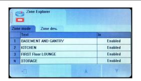
Select the Zone to Disable by pressing the "In" field. The status changes from enabled to Input Disabled.
