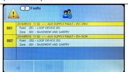
The fault message indicates whether the interface has detected an open or short circuit fault on its field wiring, or if it has lost it's auxiliary power supply input
