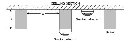
Figure 5: Smoke detector spacing — beam construction (side view)
