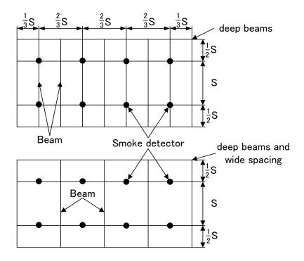
Figure 6: Smoke detector spacing — beam construction (plan view)
