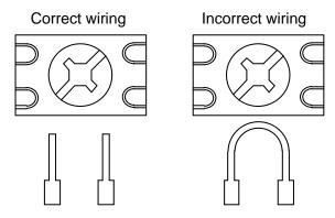
Figure 10: Correct and incorrect wiring method
