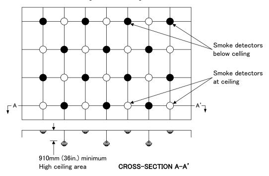
Figure 2: Smoke detector layout accounting for stratification
