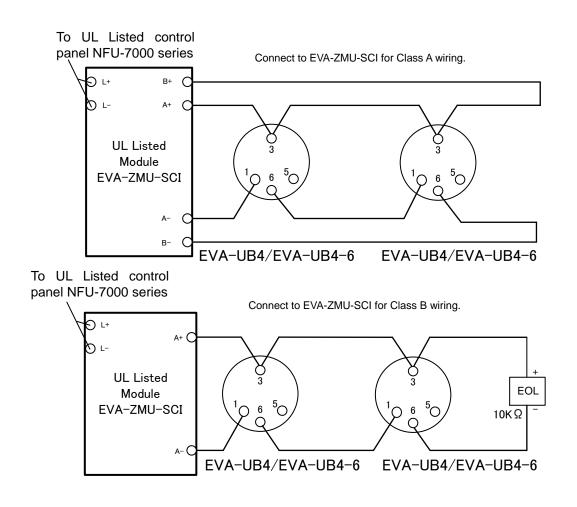
Figure 9: Wiring diagram for EVA-UB4 and EVA-UB4-6
