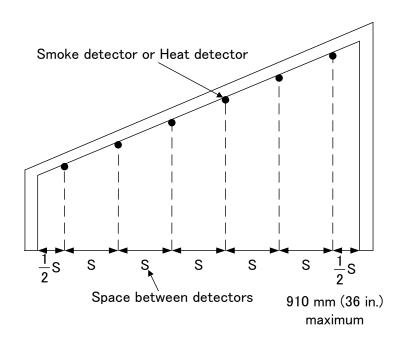
Figure 8: Smoke detector spacing — Sloped ceiling (shed type)
