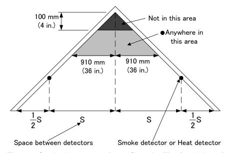
Figure 7: Smoke detector spacing — Sloped ceiling (peaked type)
