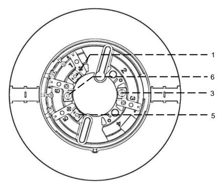
Figure 2: Position of terminals (EVA-UB4-6)
