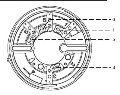
Figure 1: Position of terminals (EVA-UB4)
