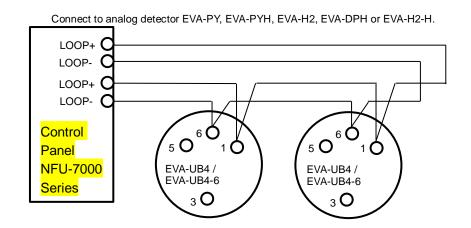
Figure 8: Connection to control panel NFU-7000 series
