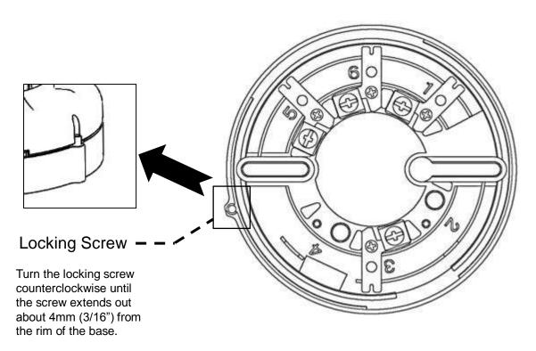
Figure 7: Position of locking screw
