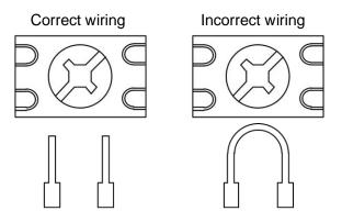
Figure 9: Connection to terminals
