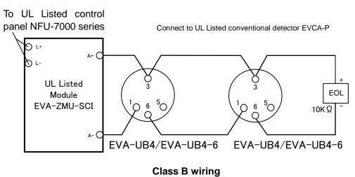
Figure 9: Connection of conventional detector EVCA-P
