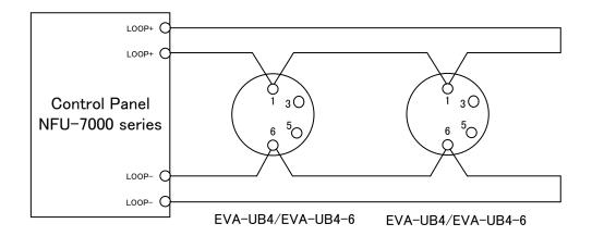
Figure 9: Wiring diagram for EVA-UB4 and EVA-UB4-6
