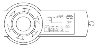
Figure A.1: Mounting a detector on EVA-AD2
