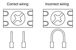
Figure 10: Correct and incorrect wiring method
