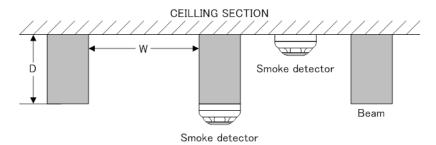
Figure 5: Smoke detector spacing — beam construction (side view)
