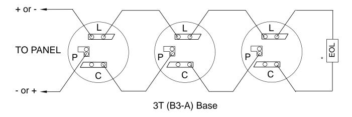
\* EOL: End of Line devices usually come with the fire alarm control panels or other devices to which the detectors connect.
