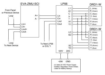
\*1 A 10 k $\Omega$  End-of-Line Resister must be installed at the last LP06 in the A+ and A- circuit.
