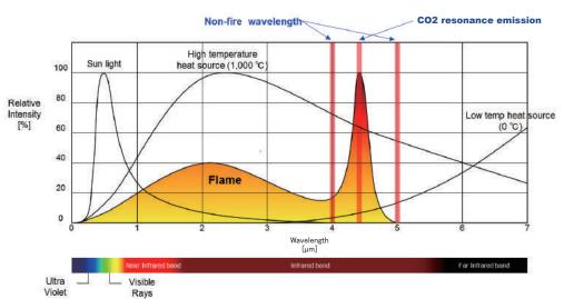
Fire (flame) has a characteristic peak at  $4.4 \mu m$  in a spectral distribution, which is called as CO2 emission. The DRD1-W has 3 sensors that monitor the band of CO2 emission and two wavebands on either side respectively. The detector avoids false alarms by the feature of frequency-fluctuation detection.
