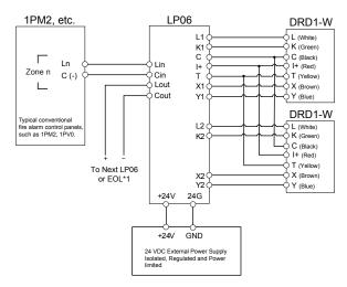
\*1 A CRE End-of-Line Device must be installed at the last LP06 in the Ln and C circuit.
